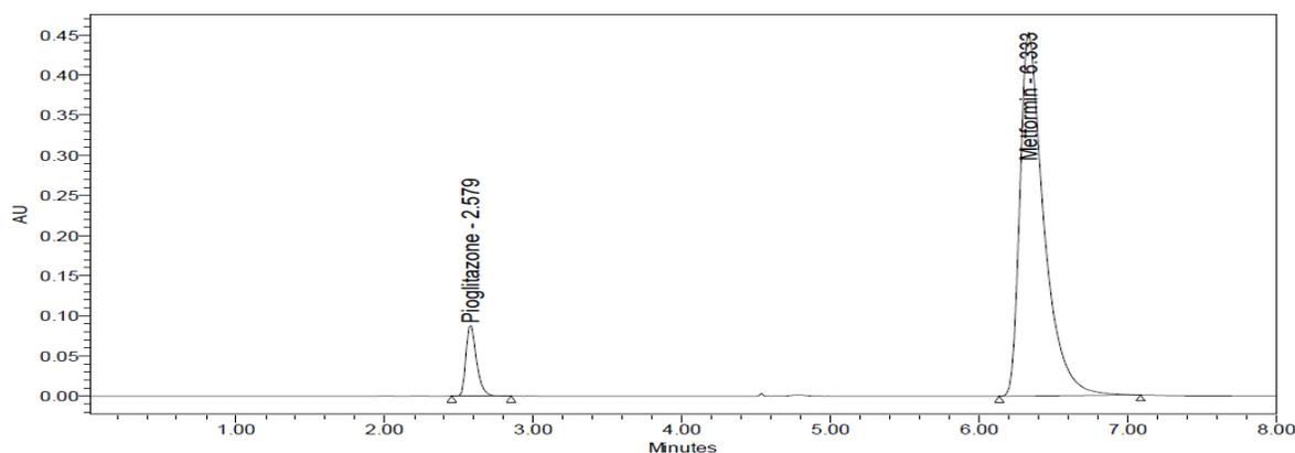
Figure-1: Chromatogram of MET (1000 $\mu\text{g/ml}$ ) and PIO (60 $\mu\text{g/ml}$ ) standard
