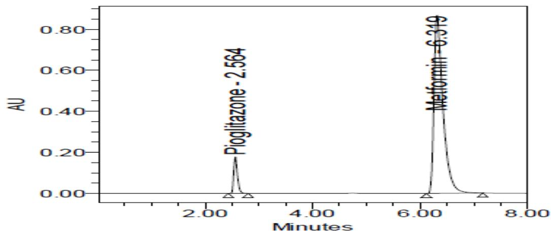
Figure-2: Chromatogram of MET (1000 $\mu\text{g/ml}$ ) and PIO (60 $\mu\text{g/ml}$ ) sample
