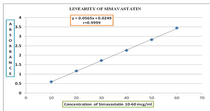
Figure 1. calibration curve for simvastatin at 238nm
