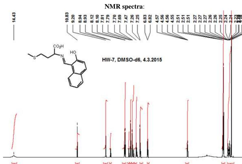
Fig 2. <sup>1</sup>H NMR spectrum of 3
