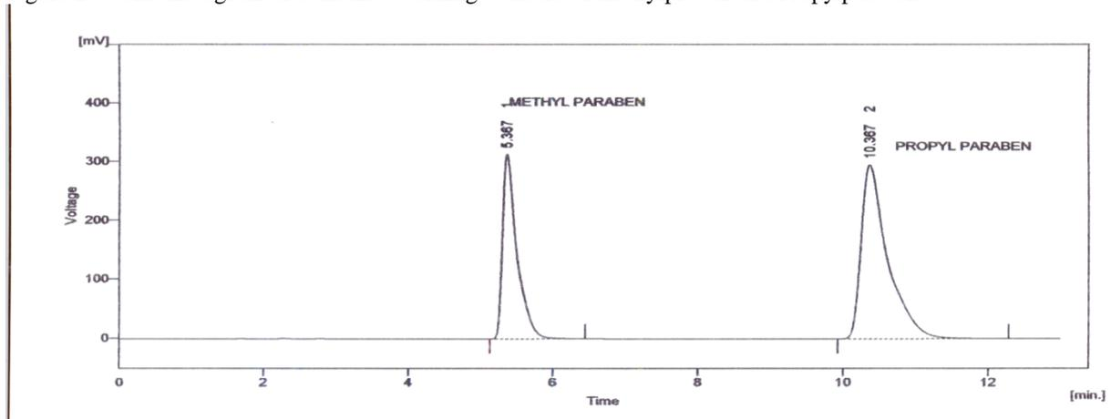
Figure 3: Standard of methylparaben and propylparaben & Placebo
