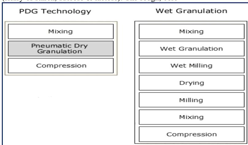
Fig.1 comparison between PDG & wet granulation
