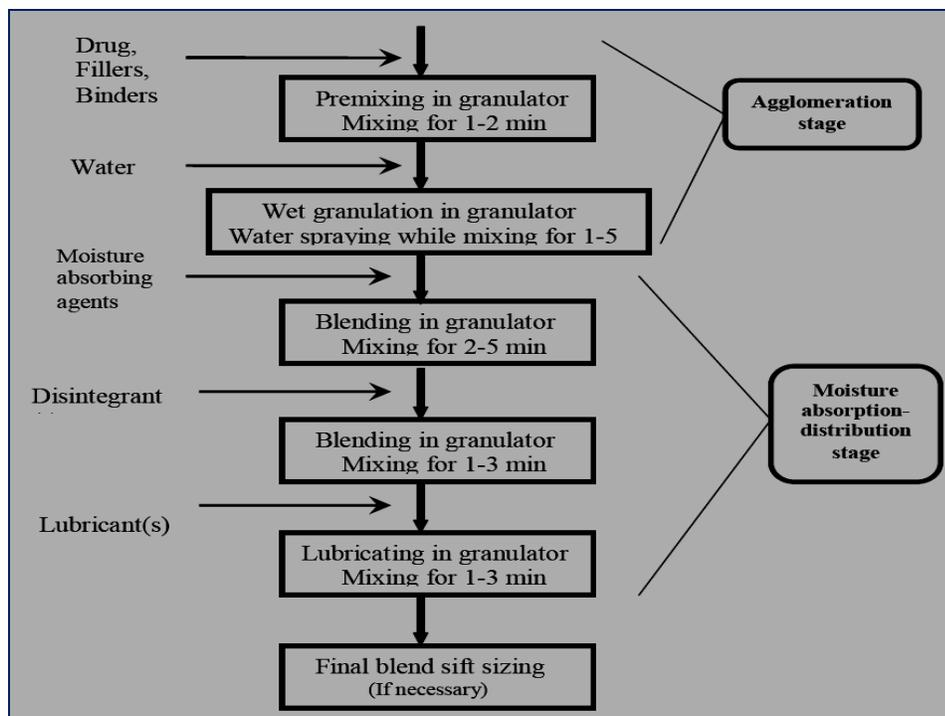
**Fig.3: Flow diagram of moisture activated dry granulation process [15, 16, 17]**
