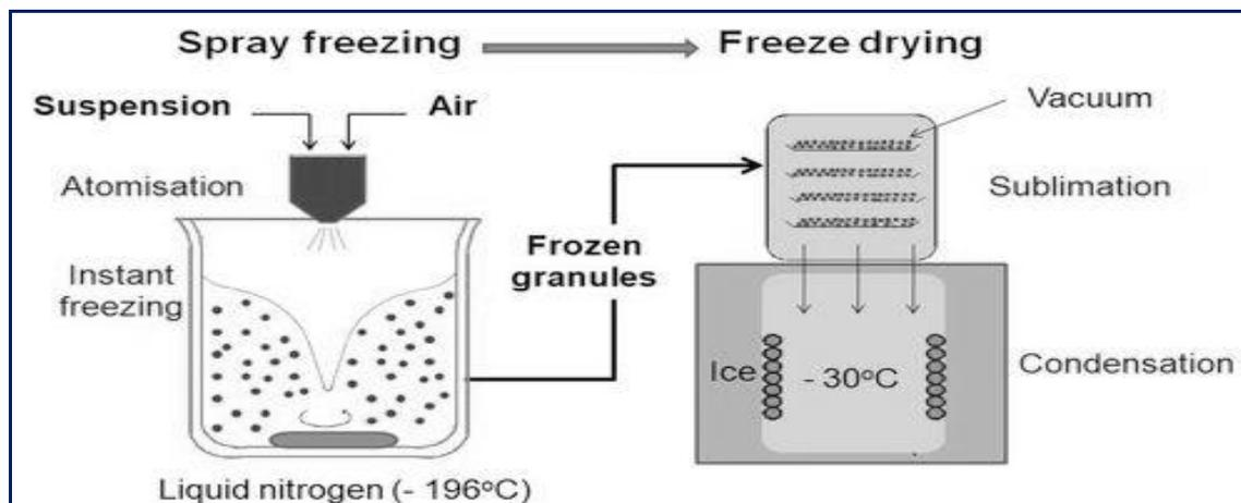
**Fig.2 Freeze Drying**
