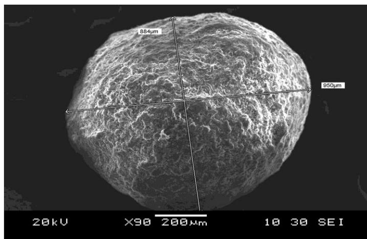
Figure 4: SEM of Venlafaxine hydrochloride pellets
