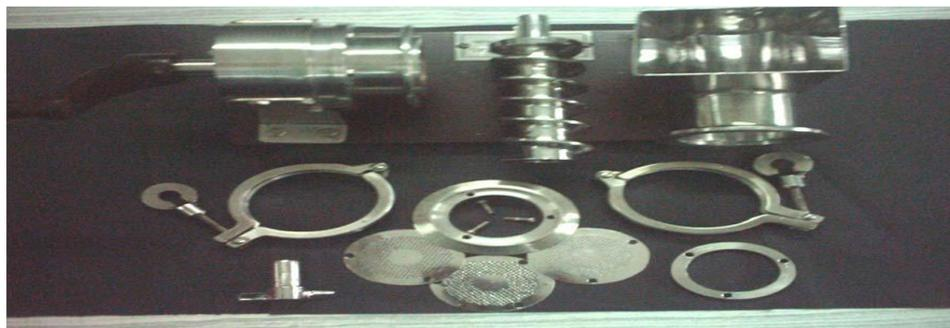
Figure 1: Parts of a Single Screw Extruder (Manual – Axial type)
